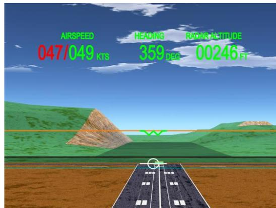
**Fig. 69: HUD used during the Decelerating Approach Task**
