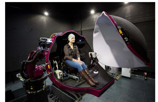
EEG signals from skin electrodes indicate the operational levels of attention and workload.
