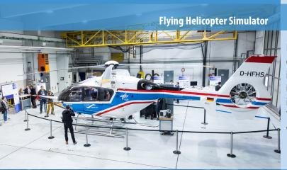
DLR's Flying Helicopter Simulator (ACT/FHS) is a modified EC135 helicopter that can simulate other aircraft in real flight. Within myCopter it was used to investigate the flight dynamics and human-machine interface of a future PAV. The cockpit was equipped with a highwayin-the-sky display and a steering wheel for intuitive car-like control. This is the first helicopter to be flown with a steering wheel. Watch a video here.
