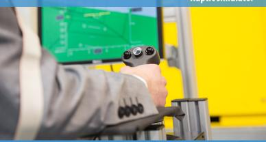
We combined a highway-in-the-sky displays with a haptic shared control framework to assist a non-expert pilot with force guidance cues during a flight through a tunnel trajectory. We have shown that this combination provides an easy-to-use control interface for flying a PAV. Participants could experience this for themselves in a fixed-base simulator. Watch a video here.
