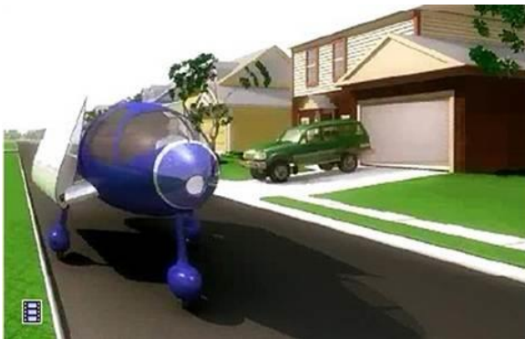
Figure 1.13: Picture of a “TailFan” vehicle with folding wings and tail, concept by NASA
