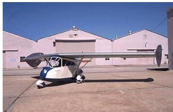
Figure 1.8: The Aerobile by Waldo Waterman. A high-wing monoplane with detachable wings and three wheels.
