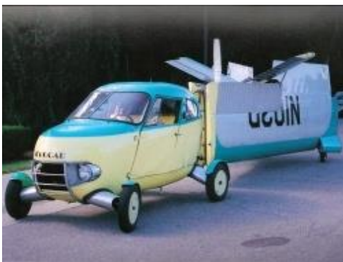
Figure 1.7: The Taylor Aerocar with foldable wings and a detachable tail unit
