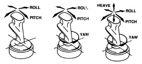
Figure 9.1a, b, c: 2DoF, 3DoF, and 4DoF controller [23]
