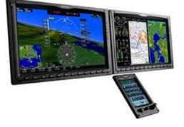
Figure 10.4: The Garmin G2000 flight deck
