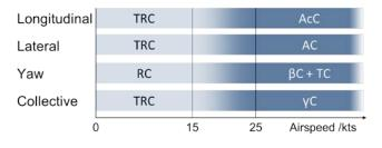
Figure 8.5: Hybrid response type configuration for PAV usage
