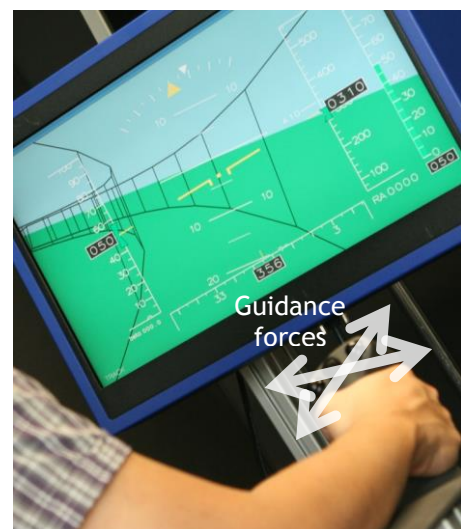
Left: An overview of a flight trajectory. Right: lateral guidance forces and velocity cues were provided to participants on a sidestick. Additionally, a collective lever was used to provide guidance forces related to the vertical changes in the flight path (not shown).
