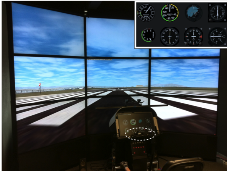
Fig. 1. Flight simulator with remote eye-tracking cameras (indicated in the white ellipse). Instrument panel is featured inset (From left to right. Top panel: RS, ASI, AI, AT. Bottom panel: TQ, CO, HI, VSI.)
