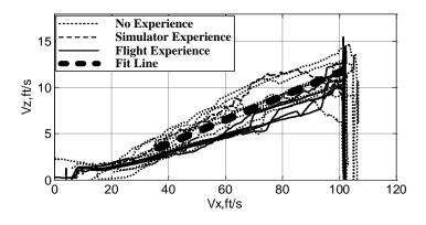
Fig. 52 Illustration of constant flight path angle in phase 2 of the approach manoeuvre
