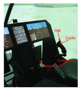
Fig. 65: Helicopter Control within HELIFLIGHT-R
