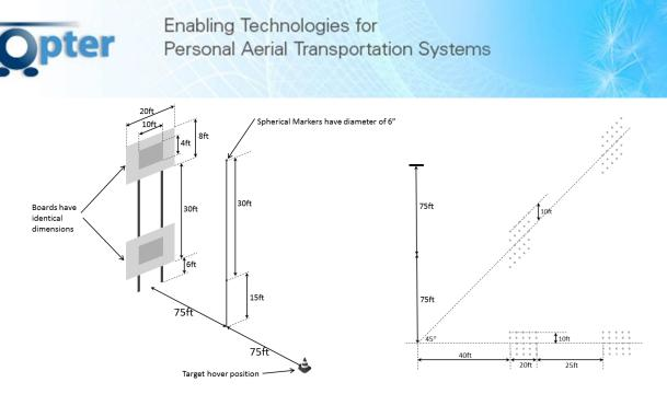
Fig. S1.2 Vertical Reposition MTE Test Course (note: ground markings are repeated to the left of the hover point)
