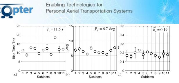
Fig. 47 Rise time, final flight path angle and coupling term values obtained from the simulated flight trials
