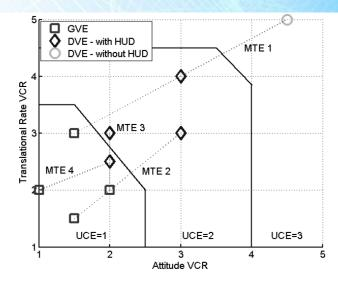
Fig. 5 Determination of UCE for Hover and Low Speed MTEs
