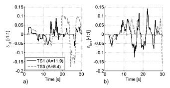
Fig. 25 Control Activity in Hover MTE with RC Configuration
