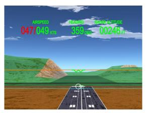
Fig. 69: HUD used during the Decelerating Approach Task
