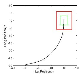
Fig. 68: Ground Trajectory for Hover Reposition Task.
