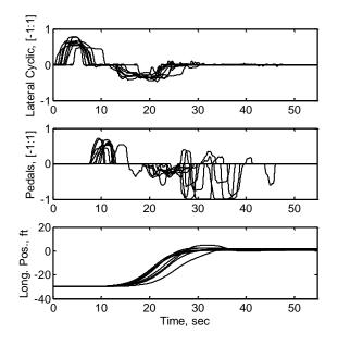
Fig. 73: Hover Reposition Task completion using nominal longitudinal control gain.
