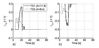
Fig. 27 Control Activity in Hover MTE with Hybrid Configuration
