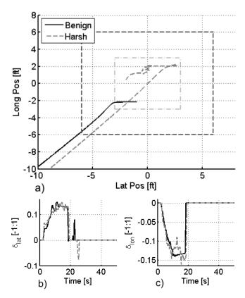
Fig. 34 Plan position and control activity in Hover MTE
