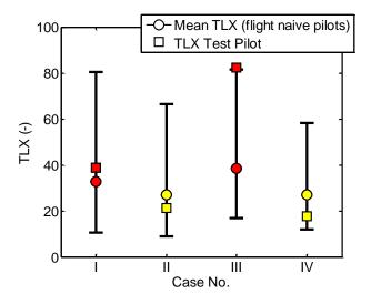
Fig. 77: Comparison between TLX Ratings for the Hover Reposition Task
