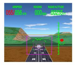
Fig. 57 Head up display used for PAV manual landing
