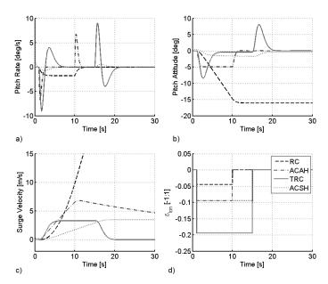
Fig. 3 myCopter PAV Model Pitch Axis Responses to Pulse Inputs
