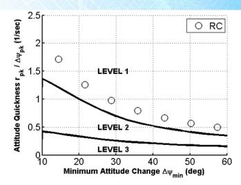
Fig. 12 Yaw Axis Attitude Quickness
