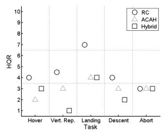
Fig. 13 PAV Handling Qualities Ratings
