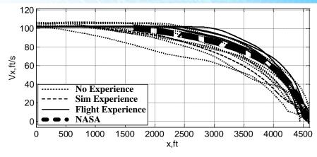
Fig. 51 Comparison of ground speed profiles between the actual data and NASA results
