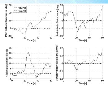
Fig. 6 Turbulence response of RCAH and ACAH configurations
