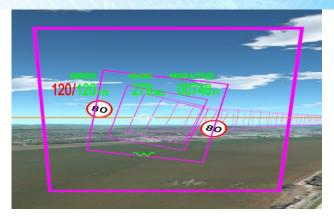
Fig. 41: Highway-n-the-Sky used for PAV Navigation
