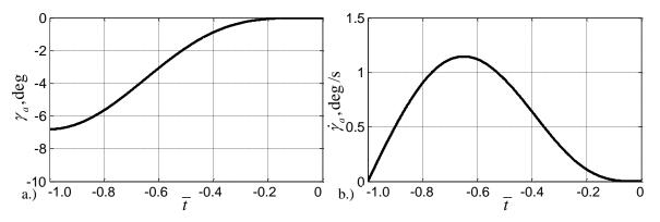
Fig. 48  $\gamma_a$  and  $\dot{\gamma}_a$  profiles derived with the intrinsic constant acceleration guide
