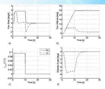
Fig. 4 myCopter PAV Model Yaw Axis Responses to Pulse Inputs
