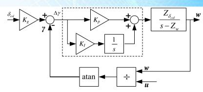
Fig. 49 Flight path angle loop with collective control ( $V_x > 25$  kts)
