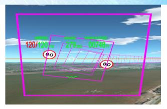
Figure 6: Highway-n-the-Sky used for PAV Navigation
