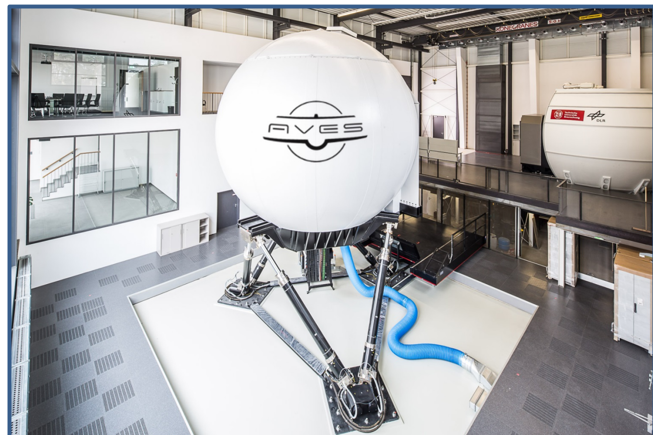
AVES motion dome in the front and fixed-based dome in the back.
