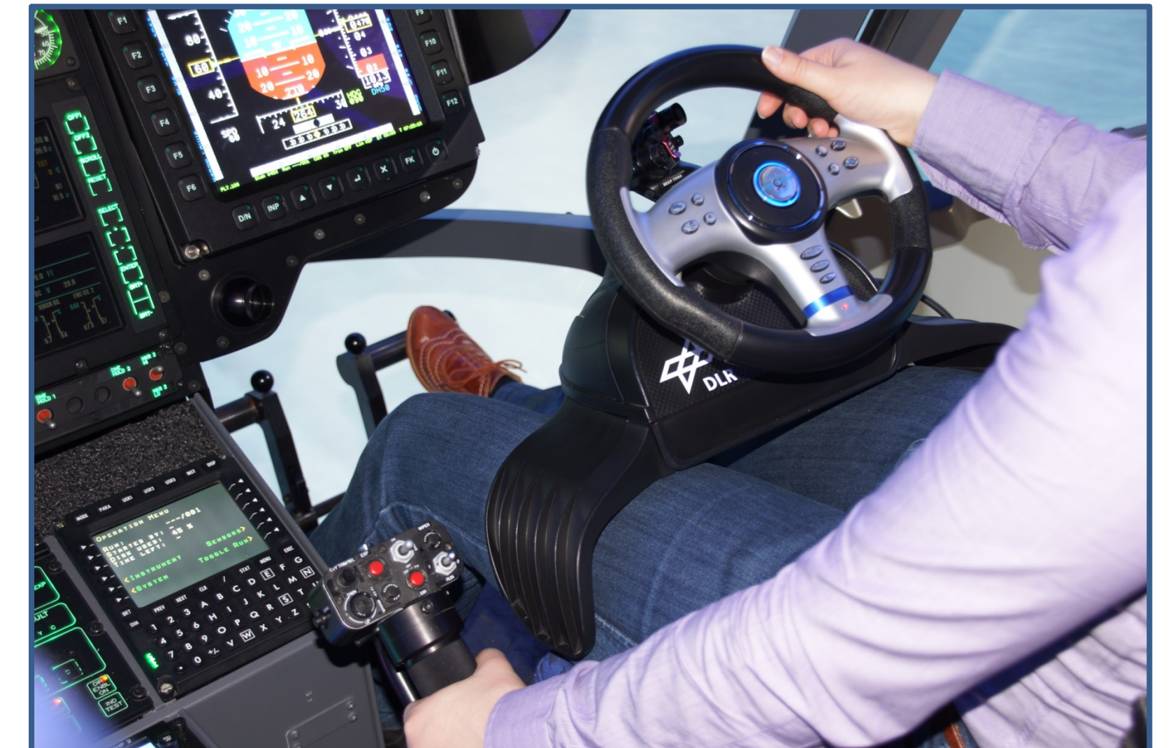
Steering wheel control for a Personal Aerial Vehicle.
