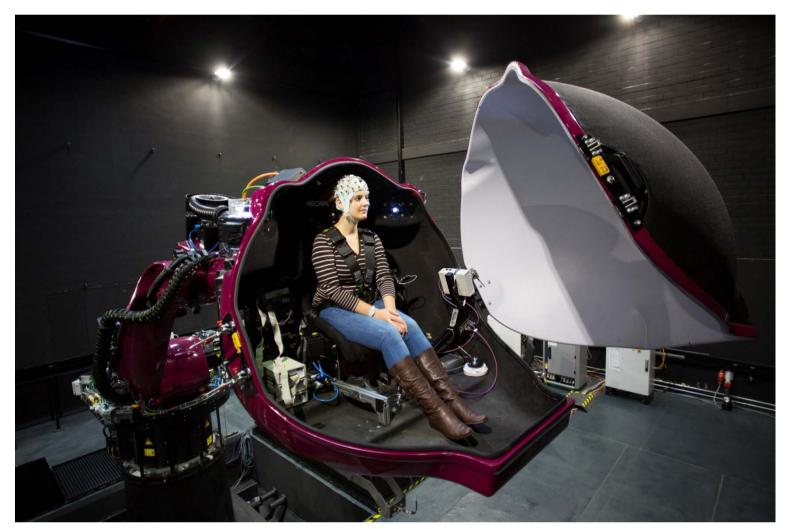
EEG signals from skin electrodes indicate the operational levels of attention and workload.
