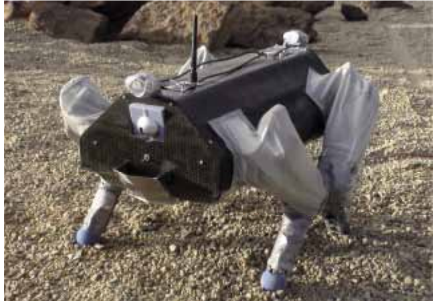
The four-legged robot a.i.f. (an autonomous walking robot with springs), which was developed at ETH Zurich, during a field trial in a crater in Tenerife. Mobile machines like this could one day explore Mars, for instance. The robots wear cuffs to protect them from dust. (Photo: ETH Zurich)
